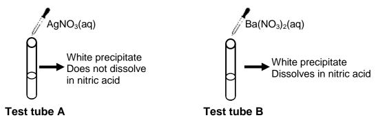
A white precipitate forms in each test tube. After addition of nitric acid, the precipitate in test tube **B** dissolves, whilst that in test tube **A** does not dissolve.
